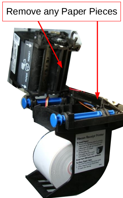
Figure 35. Removing Jammed Receipt Paper
