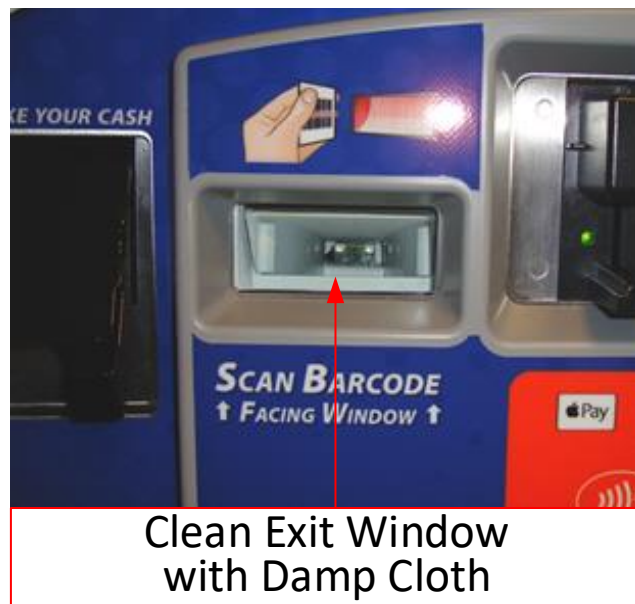
Figure 49. Cleaning Barcode Imager Exit Window
