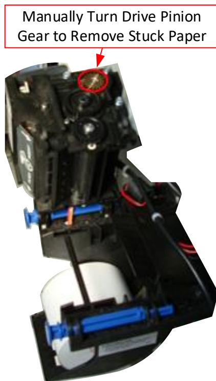
Figure 36. Manually Removing Stuck Receipt Paper
