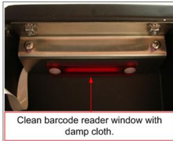
Figure 45. Cleaning the Barcode Reader Window
